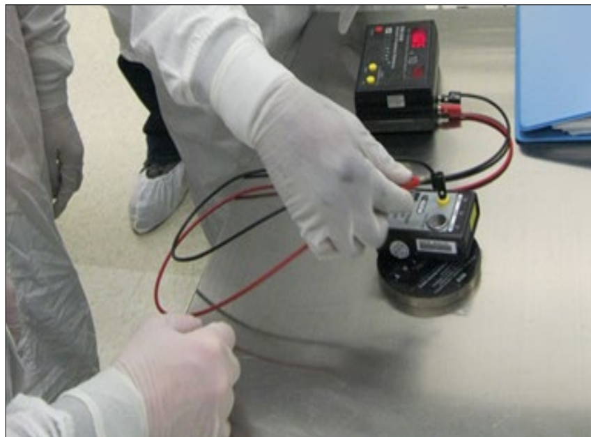
Figure E-1. Setup for Verifying Wrist Strap Checker
