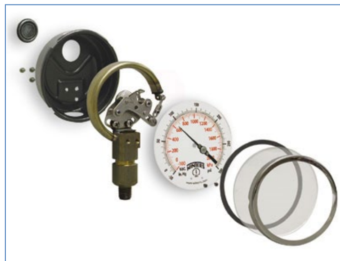
Figure 15-3, View of a bourdon-tube gauge lacking a solid front case and having a blow-out plug
